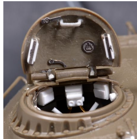
Detailed Cdr's hatch and cupola interior.
